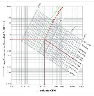
Example: for a 5 in. (125 mm) EG2 hose with airspeed of 2950 FPM (15 m/s), the pressure drop per inch per 100 feet is 6 and air volume is 350 CFM (10  $m^3/m$ ).
